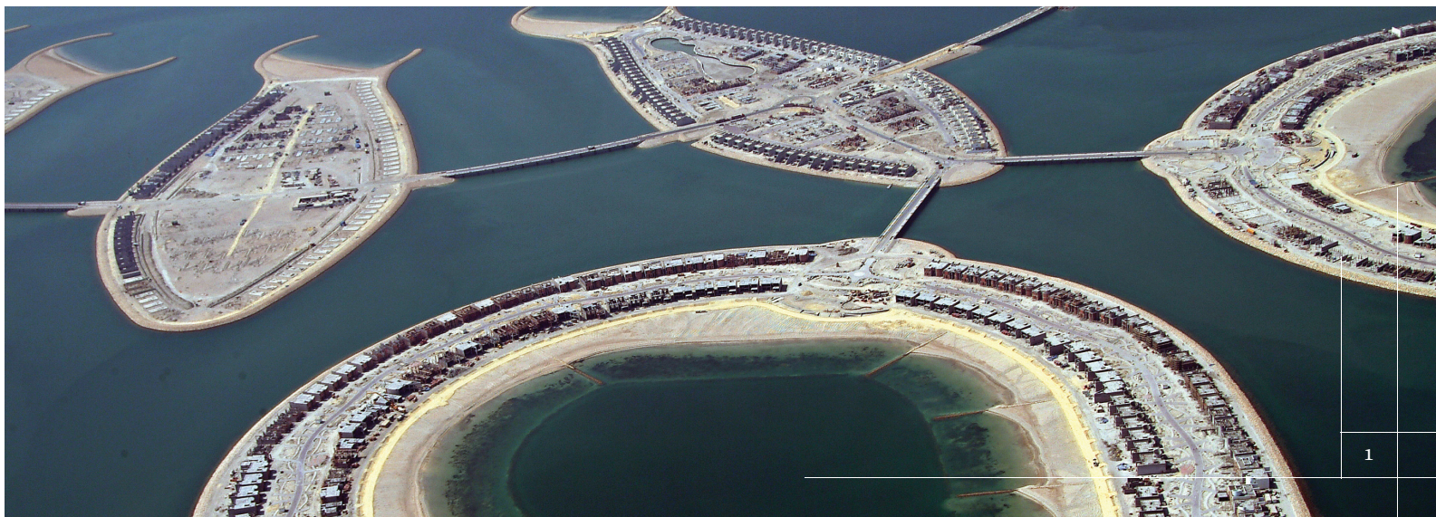
Great Lakes completed the dredging in 2007, having placed over 35 million cubic meters of sand to create 15 islands spanning 220 million square feet.
